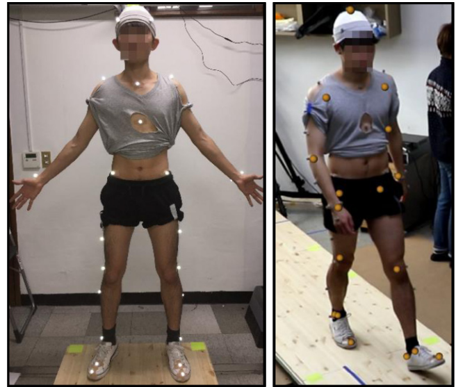
Fig. 1 Motion capture data were obtained during walking (left). Three-dimensional anatomical joint positions were calculated and re-projected onto video frames (right)
