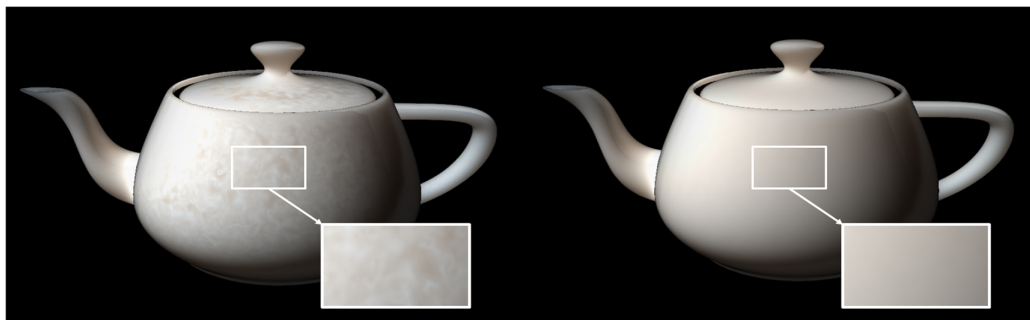
Fig. 9 Accuracy comparison of the approximation results between the LPF based wavelet (left) and the non-linear wavelet (right).
