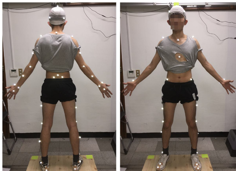
Fig. 1. Forty-three retroreflective markers were attached to the anatomical landmarks of each subject and their positions were recorded using a motion capture system.
