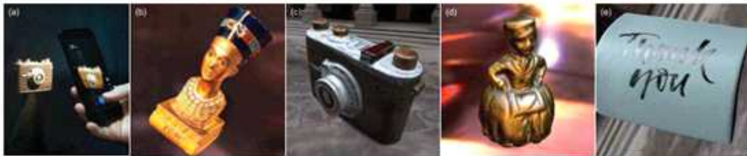
Fig. 1. We propose a practical method that enables us to capture spatially-varying BRDFs from unstructured flash photographs . It yields high-quality SVBRDFs, as well as detailed geometry of 3D objects, without relying on any expensive supporting hardware nor controlled illumination, using instead any hand-held conventional digital camera with a built-in flash. No input geometry is needed in our algorithm. Image (a) shows our acquisition setup, while (b) – (e) show example results of our reconstructions.
