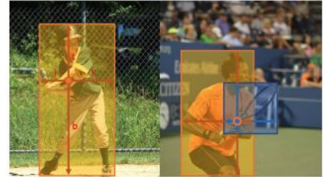
Figure 1 – As shown in the left image, FCOS works by predicting a 4D vector (l, t, r, b) encoding the location of a bounding box at each foreground pixel (supervised by ground-truth bounding box information during training). The right plot shows when a location residing in multiple bounding boxes, it is ambiguous in terms of which bounding box this location should regress.
