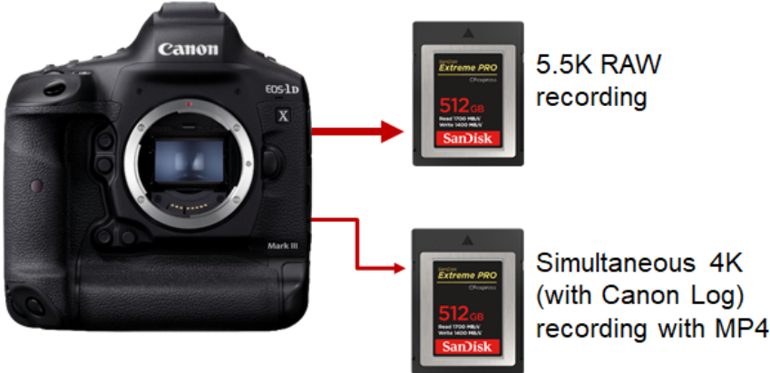
Figure 8 Simultaneous recording of the Master 5.5K RAW and an MP4 4K format
